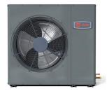
The XR16 Low Profile Heat Pump from Trane is a side-discharge, single-stage heat pump designed for split ducted heating and cooling systems where space constraints make vertical discharge units difficult to install. It is available in 1.5 to 5 tons and is suitable for any residential building. The
